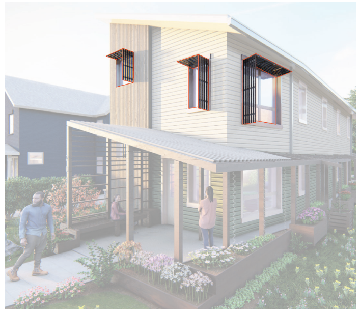
Shading Devices (West and South-west facade)
